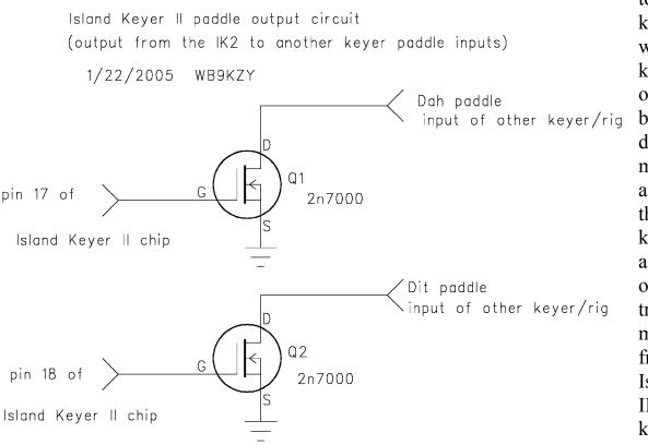
another to kever or rig with a built in keyer. These outputs will be actuated during a memory play and will "key" the external kever. This allows the operator to transfer memories from the Island Kever II to another keyer. One user who was
