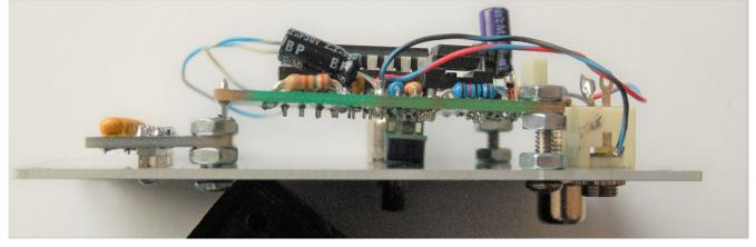
Then with the remaining two 4-40 nuts the right side can be secured and the header soldered.
