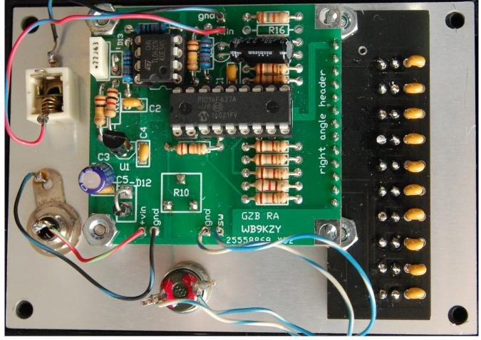
5) Finally (after testing it out) mount the board in the case using the 4 black 4-40 machine screws.
