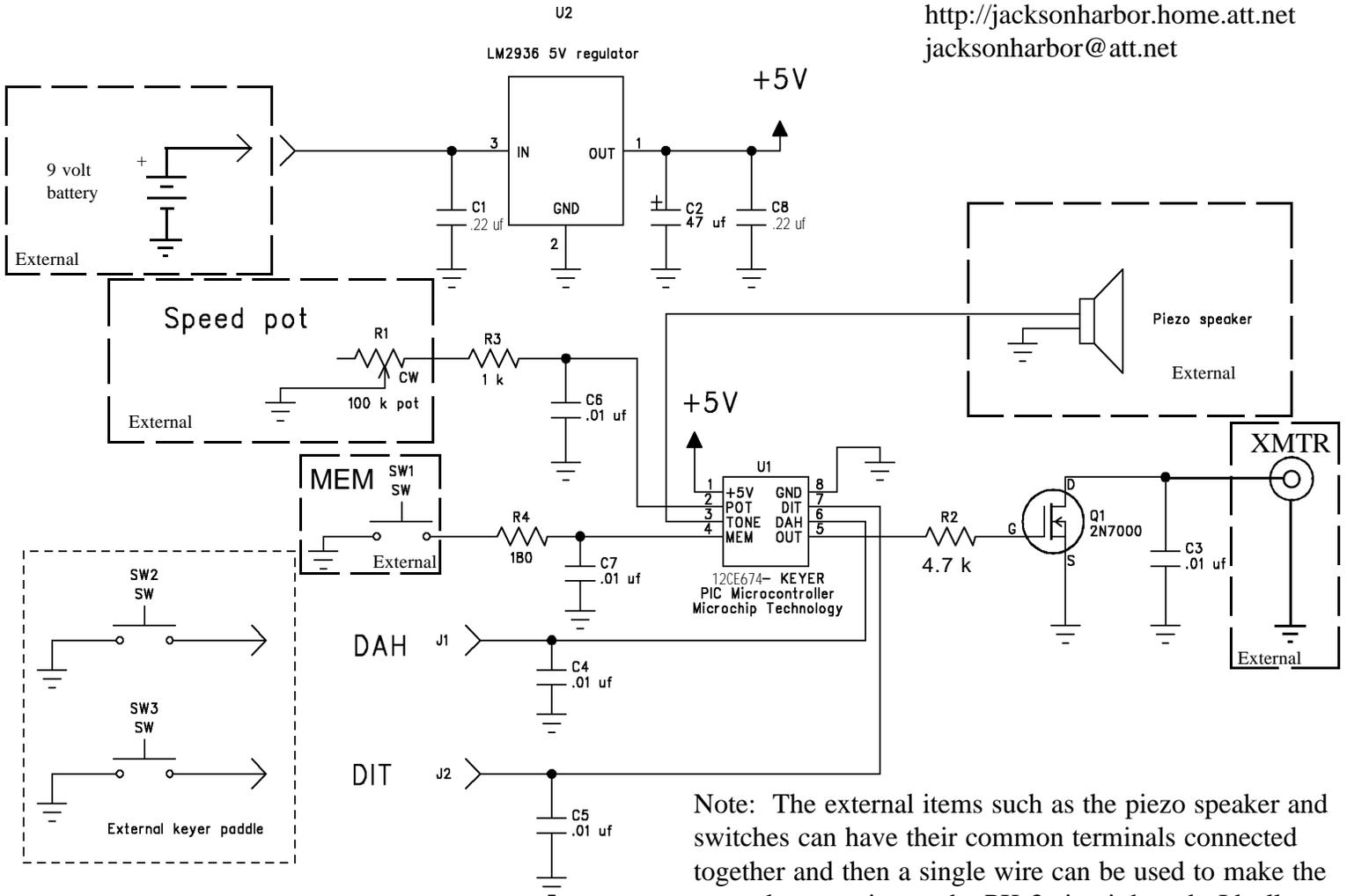
Note: The external items such as the piezo speaker and switches can have their common terminals connected together and then a single wire can be used to make the ground connection to the PK-3 circuit board. Ideally, the PK-3 will be housed in a metal case - the board mounted with a short metal standoff and star washers to insure a good electrical connection to ground.
